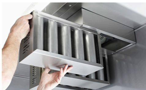
A filter cassette consists of ten cyclones. The cassettes are easily removed for cleaning in the dishwashing machine
